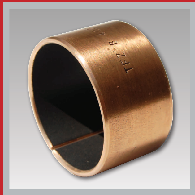
WRAPPED COMPOSITE SLIDING BEARING, BRONZE/PTFE, MAINTENANCE-FREE
